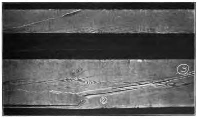
Fig. 29.—Failure due to spiral grain. Views of side and bottom of central portion of  $8'' \times 16'' \times 16'$  stringer after test. It will be noted that the lines of failure do not follow the visible grain (lines formed by cutting the annual rings).
